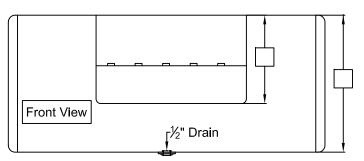
Please note: All sizes are NPTF unless otherwise noted and reference all measurements from the lateral weld seam and the end cap weld seam to the center of the fittings.
